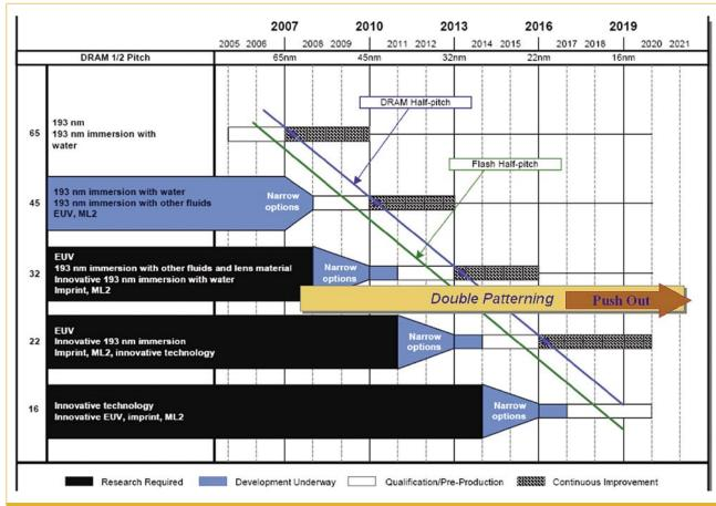
Figure 1. The ITRS 2005 roadmap insertion of a new 'double patterning' element to gain development time for EUV.
