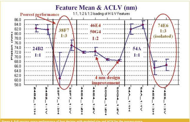
eliminated the random metrology and exposure noise contribution and can directly measure the sensitivity of the feature-design aberrational response at each process-exposure.
