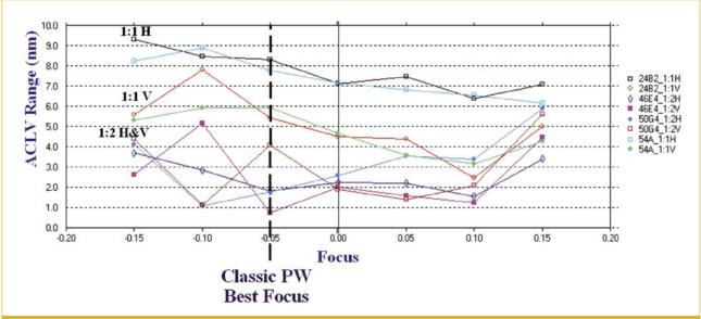
Figure 5. ACLV design response at 25mJ/cm<sup>2</sup> for varying defocus of 1:1 and 1:2 loaded 70nm features. Classic techniques suggest optimum focus to be located at -0.05um but ACLV is minimized if +0.05um is used.
