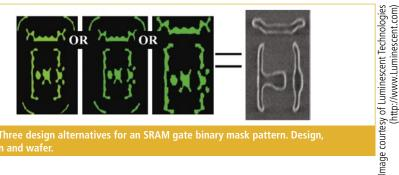
Figure 2. Three design alternatives for an SRAM gate binary mask pattern. Design,
